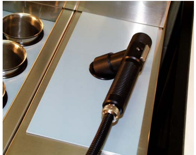
A close up view of the filling gun used by the operator for filling the beakers and for topping up the Mash with a specific volume of d/water during a cycle.
