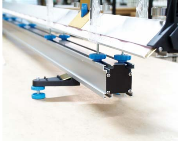
AIR TRACK WITH SUB BASE FITTED
