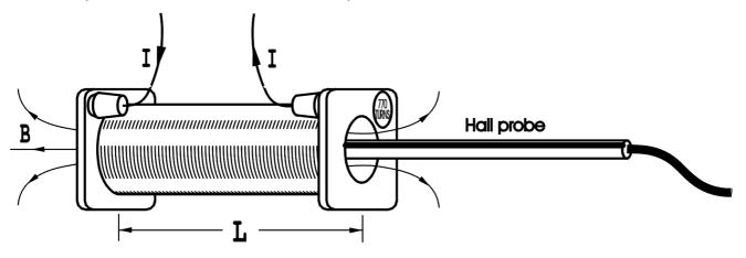
Select Constant Current meter to read amps and connect the solenoid and adjust the current through the solenoid to exactly 1.7 amp. Use the equation:
