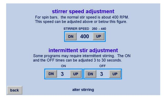
This display permits the adjustment of stirrer speed and the intermittent stirring time, when programmed.
