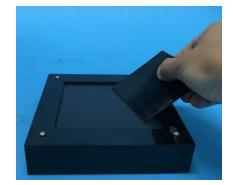
$\leftarrow$  Frost on the cold plate surface is being removed.
