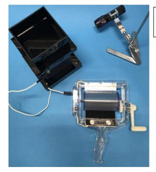
Connecting the cable from the minus terminal of Static Genecon to the screw of the hot water tub.
